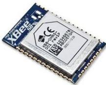
The 868/915 MHz frequency band is mostly used for applications requiring a larger range. The Xbee 868LP [38] module is an example of a solution applying the 802.15.4 standard in this frequency range. It can transmit up to 112 meters indoors or 8.4 km outdoors, but has relatively small maximum data rates, only up to 80 kbps, compared to Bluetooth 5.0.
