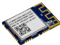
Microchip’s ATWINC1510 [35,36], an example COTS product using the 802.11n standard, “is a low-power consumption 802.11 b/g/n IoT module, which is specifically optimized for low-power IoT applications”. This module consumes 61 mA when transmitting @ 6 Mbps, which is 6 times more compared to a Bluetooth 5.0 solution. However, a 6 Mbps or even 54 Mbps data rate will likely be more than needed for usage in I-MECH Layer 1, where data is likely transmitted between only a few sensors.
