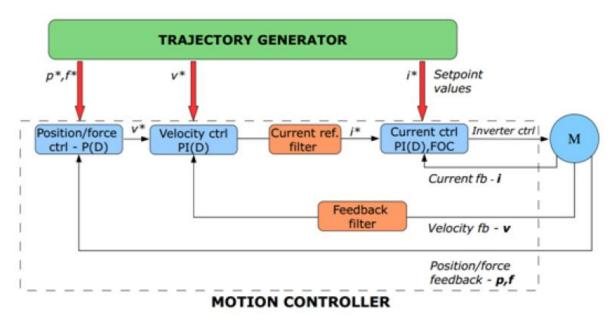
Figure 3.5: Three level cascade control structure
