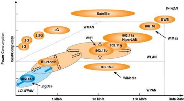
Figure 3.4: Wireless standards compared in terms of data rate and complexity of implementation [22].
