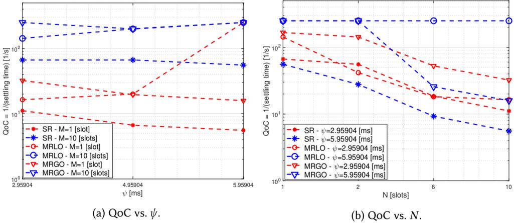
Fig. 11. Impact of  $\psi$  and  $N$  to the system output for the SR, MRLO, and MRGO design flows. (a) Fixed  $N = 10$  slots, varied  $\psi$  with 2.95904, 4.95904 and 5.95904 ms, and varied  $M$  with 1 and 10 slots. (b) Fixed  $M = 1$  slot, varied  $N$  with 1, 2, 6, and 10 slots, and varied  $\psi$  with for 2.95904 and 5.95904 ms.
