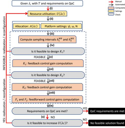
Fig. 7. MRLO design flow. The control design is highlighted within the dashed box.
