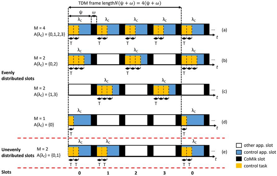
Fig. 3. Resource allocation examples for application  $\lambda_C$ , using a TDM frame with  $N = 4$  slots. Top (a,b,c,d): evenly distributed application slots. Bottom (e): unevenly distributed application slots - this allocation is not allowed in the remaining of the paper.
