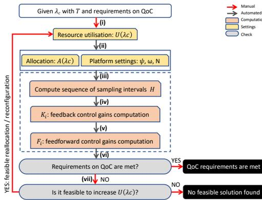
Fig. 8. MRGO design flow. The control design is highlighted within the dashed box.
