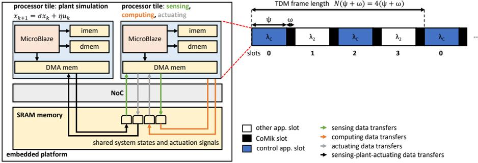
Fig. 1. Left: example of a TDM-based execution platform. Right: example for  $N = 4$ , with applications  $\lambda_C$  and  $\lambda_2$  (where  $\lambda_C$  is the control application). The black blocks indicate the CoMik slots while the blue and white blocks indicate the application slots for applications  $\lambda_C$  and  $\lambda_2$ , respectively. The TDM frame repeats infinitely. The numbers below the TDM frame denote the slots, which are indexed from 0 to 3.
