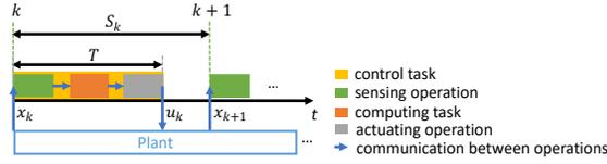
Fig. 2. Timing diagram of the control application.
