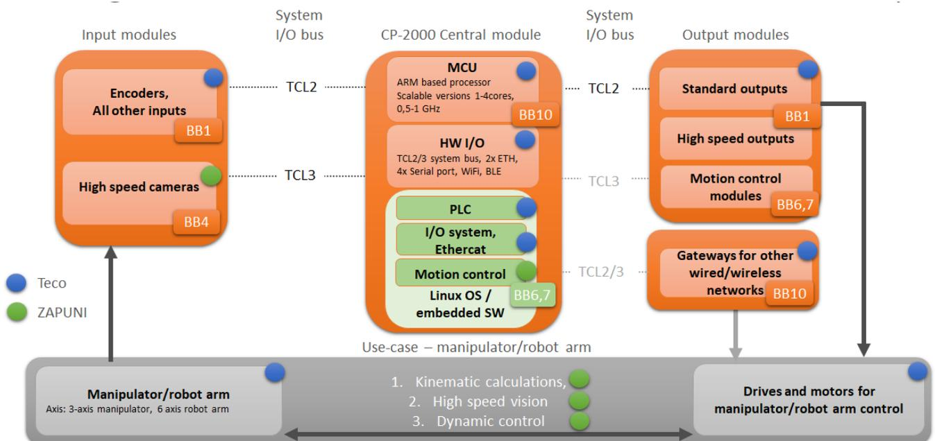
Figure 3.3.1 - Functional diagram PAC base hardware
