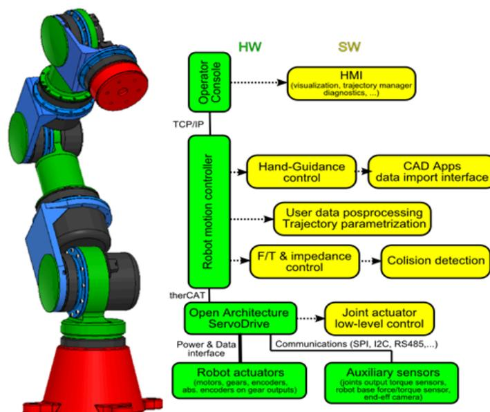
Figure 3.4.2 - Concept of open modular robotic arm
