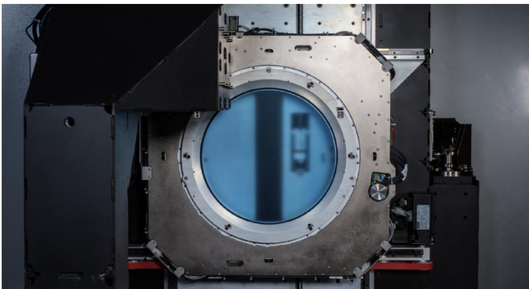
Figure 4.2.1 - Photo of the wafer stage
