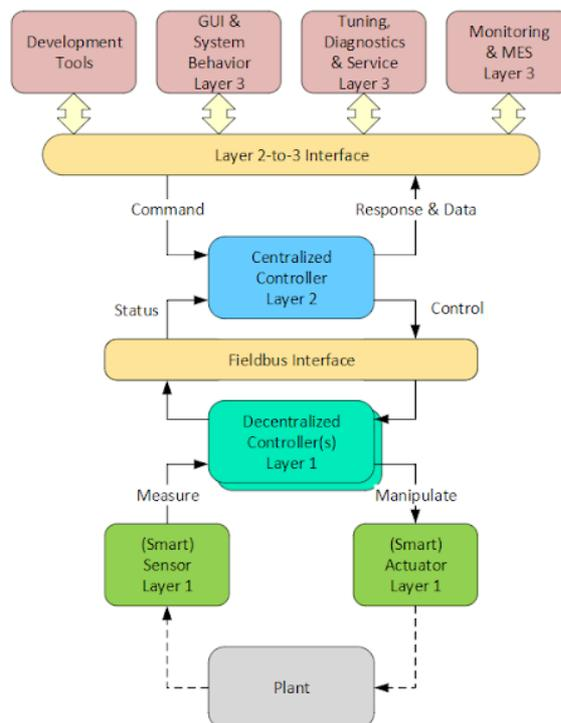
Figure 1 - Generic I-Mech motion platform model
