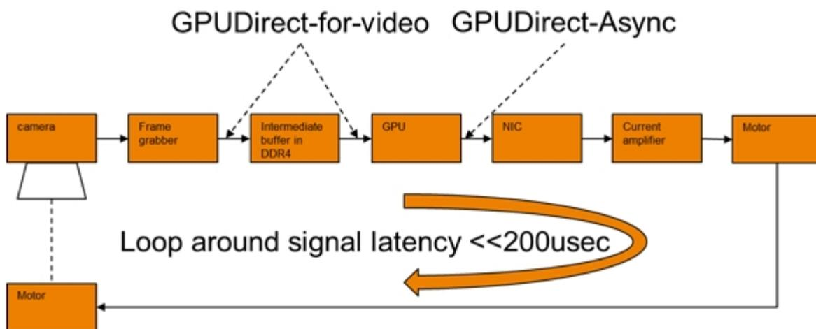
Figure 6.4.1 closed loop position control with camera over GPU
