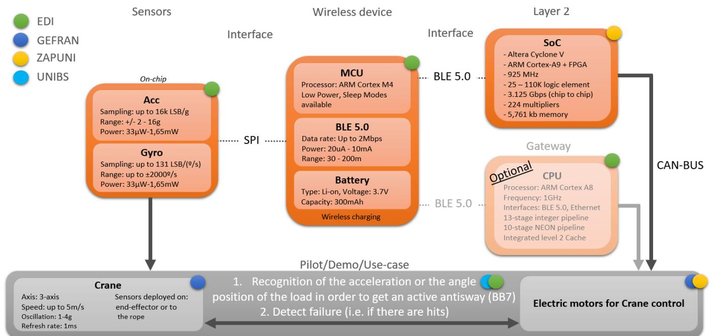
Figure 3.1.1 - Real-time wireless active anti-sway system
