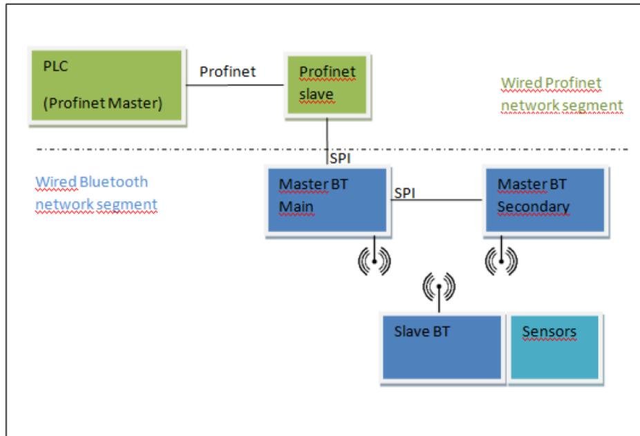
Figure 4.4.5 - Preliminary sketch of the wireless network designed in order to transfer the data collected from the sensors to the PLC of the milling machine.
