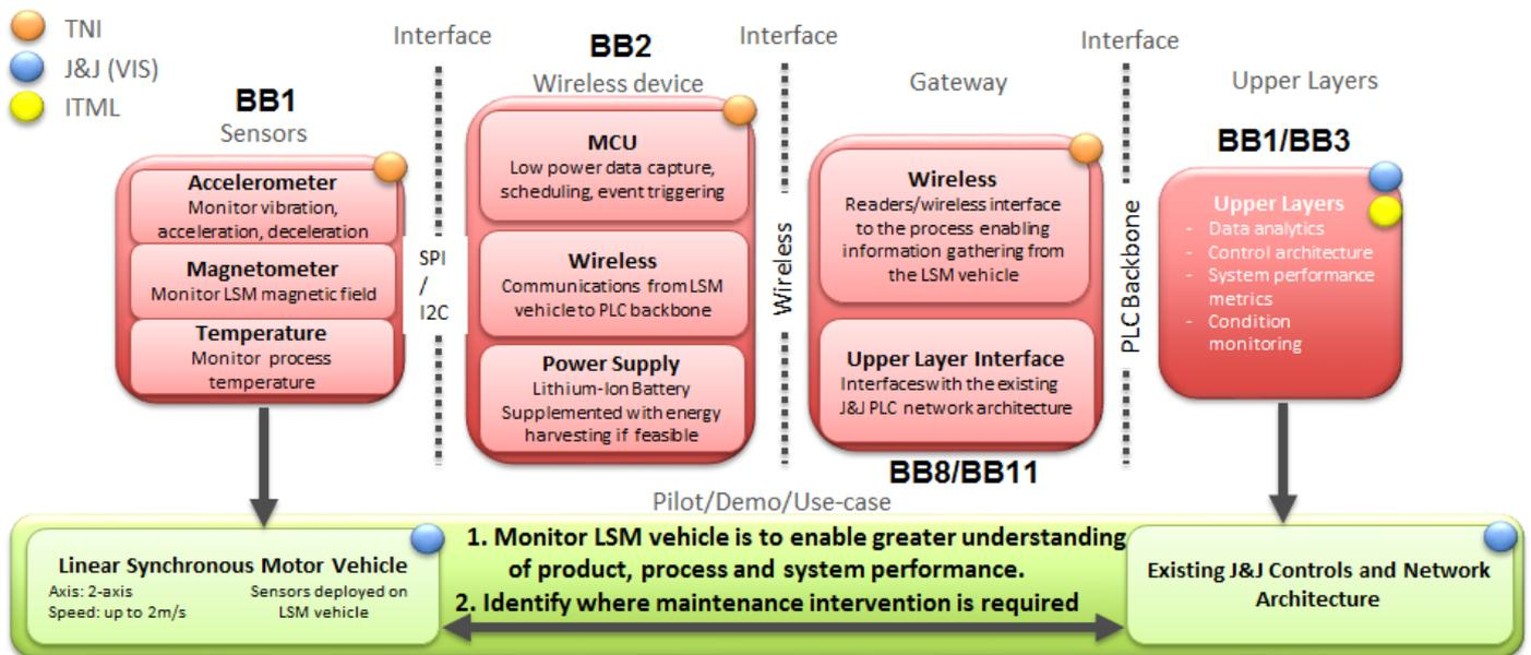
Figure 5.1.1 Condition monitoring platform for Linear Synchronous Motors (LSM) material transfer layer
