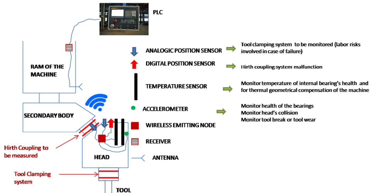
Figure 4.4.2: Illustration of how the I-MECH platform will work once integrated in the mechatronic system.
