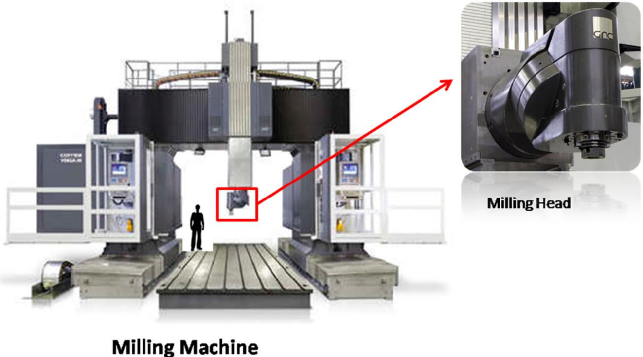
Figure 4.4.1: Example of milling machine and milling head where the I-MECH platform will be integrated in order to monitor important process parameters.
