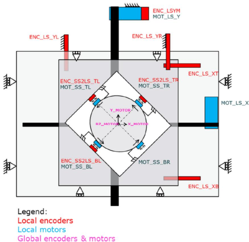
Figure 4.2.2: overview of the motors and encoders
