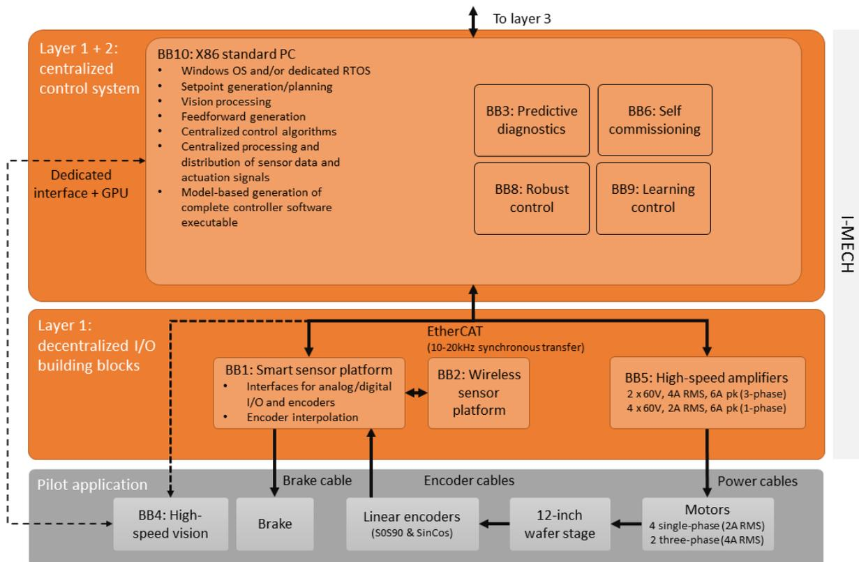
Figure 4.2.3: 12-inch wafer stage motion control
