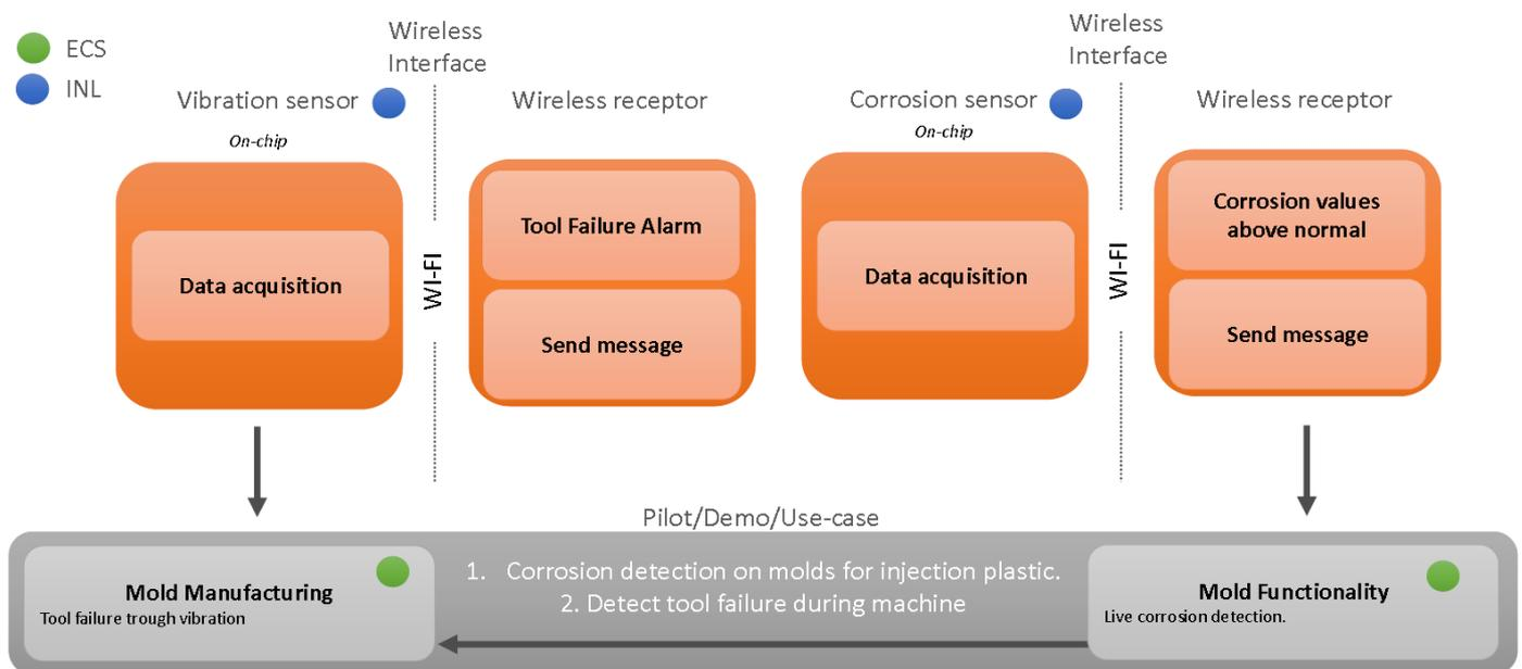
Figure 5.2.1 - Condition monitoring platform for the Injection Mold Tool.
