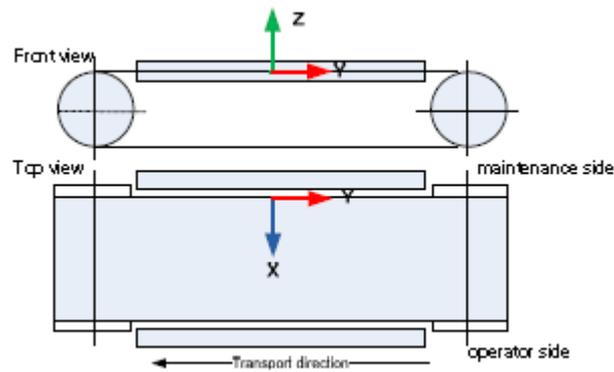
Figure 4.1.1: Direction definitions in a schematic side view of the GSC (above) and a top view of the GSC (below).
