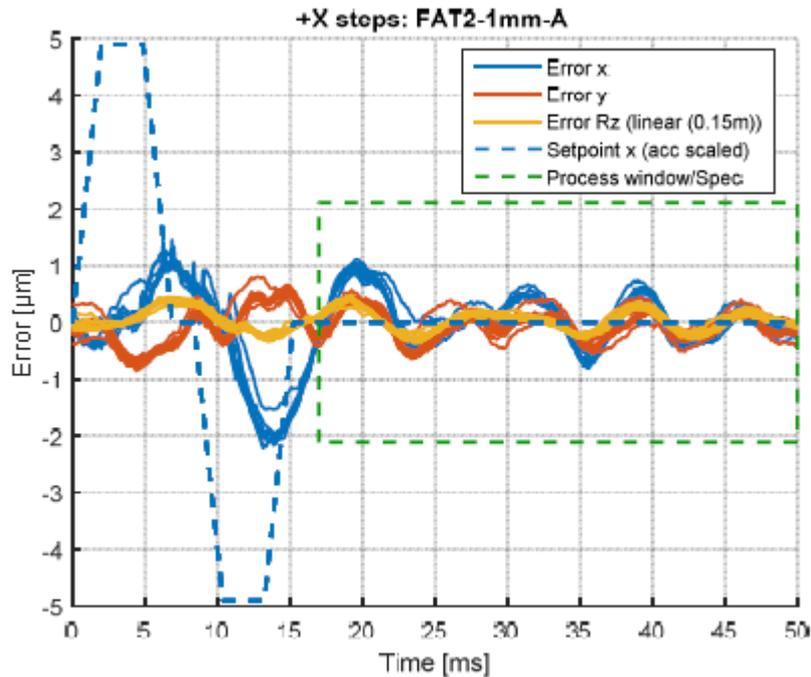
Figure 4.2.4 - Graphical depiction of 12-inch wafer stage settling requirements
