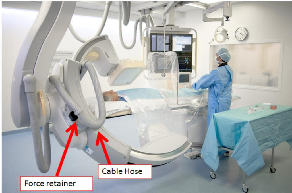
Figure 5.1.1: Cable hose and force retainer – input for model-based control
