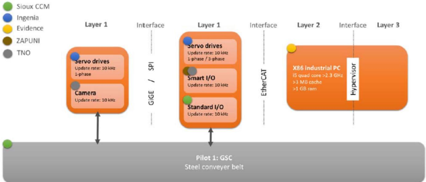
Figure 4.1.3 - Block diagram of the steel conveyor belt application
