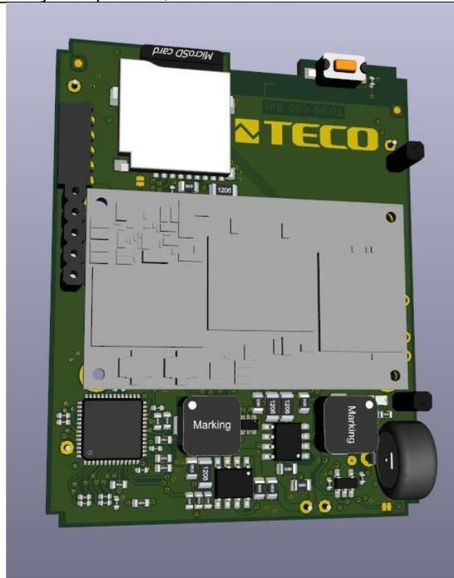
Figure 29 Design of upgraded motion control HW produced by Teco
