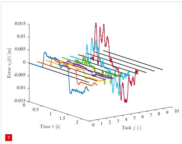
Learning from past data in a printer system using a simplified printer model (infinite belt stiffness), leading to growing error signals for subsequent tasks. At iteration 7, safety measures necessitated a shutdown of the system.
