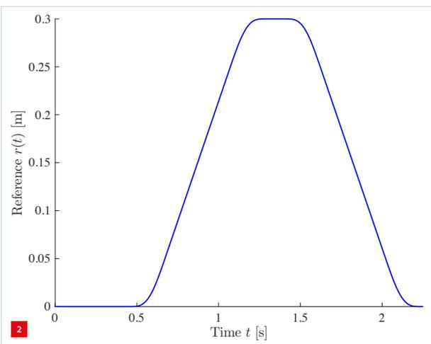
Reference for the carriage containing the printheads.
