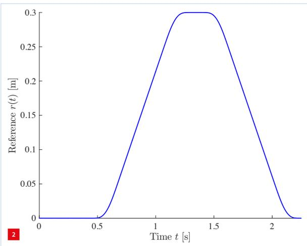
Reference for the carriage containing the printheads.
