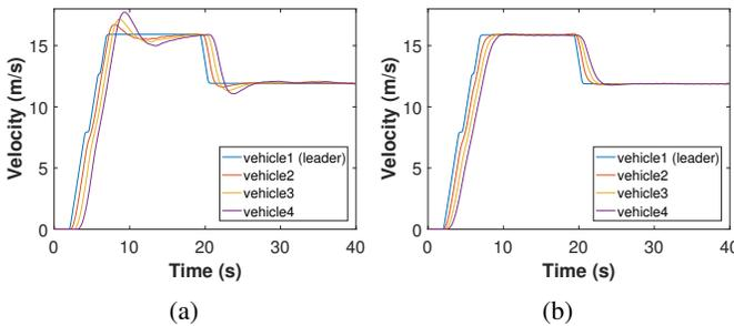
Fig. 1: The velocity response of each platoon member in two simulations. (a) String unstable (disturbance amplification). (b) String stable (disturbance attenuation).
