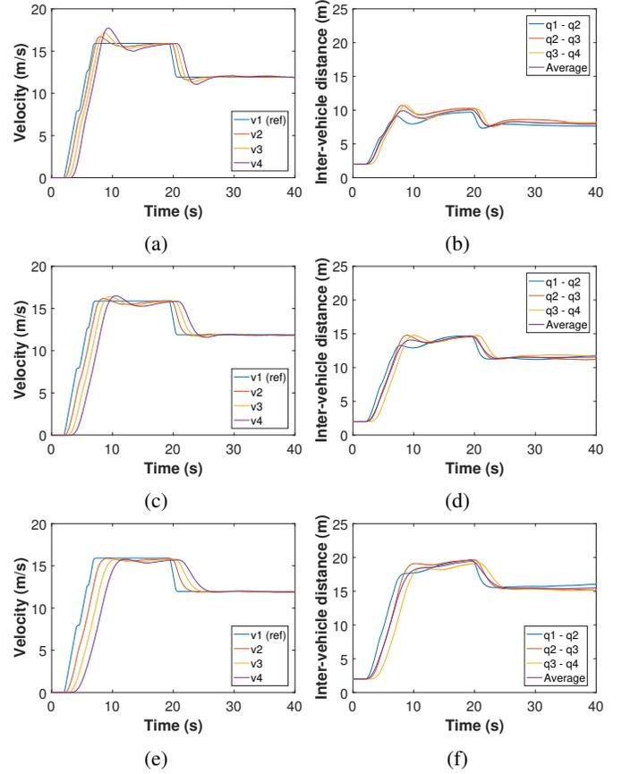
Fig. 6: String behavior with an increased headway with 2 Hz message rate: (a)(c)(e) velocity response of the platoon vehicles for 0.5 s, 0.8 s, and 1.1 s headway; (b)(d)(f) inter-vehicle distance for 0.5 s, 0.8 s, and 1.1 s headway.
