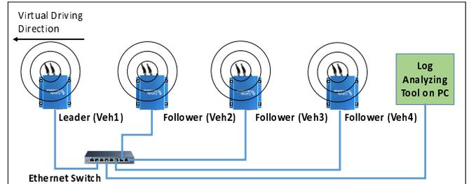
Fig. 4: Experimental setup with four MK5 nodes (1 leader + 3 followers).
