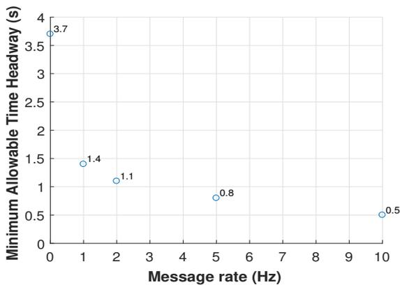
Fig. 7: MinATH for common message rates in V2X communications. (0 Hz stands for ACC).
