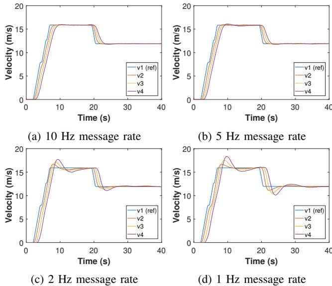
Fig. 5: CACC performance with 0.5 s time headway under different message update rate.
