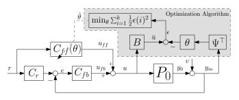
Fig. 2. Combined framework for feedforward control and parameter optimization.
