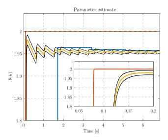
Fig. 4. Online parameter estimates, i.e.,  $\theta^{\text{noise}}$  with noise (-) with 99.7 % confidence interval (-), without noise  $\theta^{\text{noise-free}}$  (-) and the true parameter  $\theta_0$  (- -). Batch-wise estimate is also provided (-). A zoom for  $t \in [0.04, 0.2]$  shows the convergence of  $\theta^{\text{noise-free}}$ .
