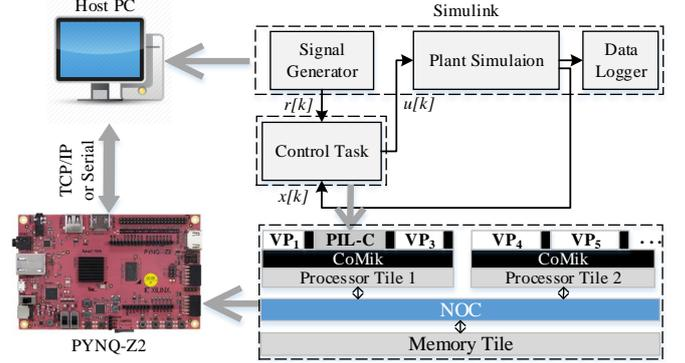
Fig. 4. PIL-C configuration. The embedded platform is implemented on a PYNQ-Z2 FPGA board. The host PC which runs Simulink communicate with the board through TCP/IP or serial connection sending  $r[k]$  and receiving the resulted  $u[k]$ .
