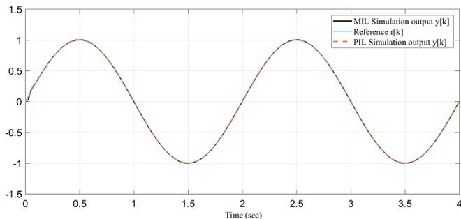
Fig. 8. PIL simulation output for PIL-C configuration. The MIL and PIL results are identical in this configuration
