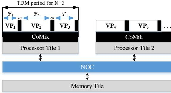
Fig. 1. Predictable embedded platform under consideration
