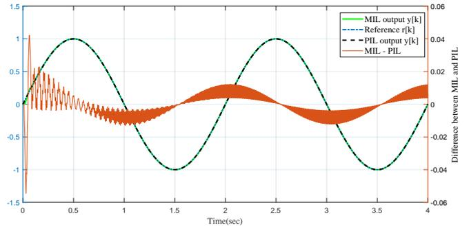
Fig. 9. PIL simulation output for PIL-CP configuration. The left hand scale is for simulation outputs and the right hand scale is for the difference between MIL and PIL simulations.
