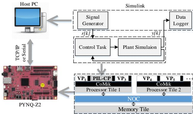
Fig. 5. PIL-CP configuration. Both control task and plant simulation are simulated on the platform. The host PC which runs Simulink communicate with the board through TCP/IP or serial connection sending  $r[k]$ , and receiving the resulted  $y[k]$ .
