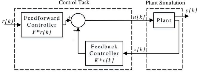
Fig. 2. 2-DOF feedback-feedforward tracking control structure
