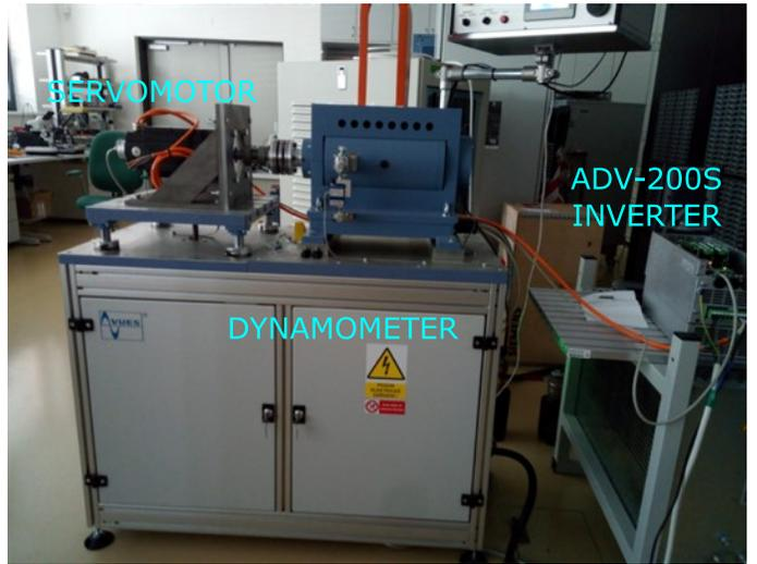
Fig. 6. Laboratory setup for verification.
