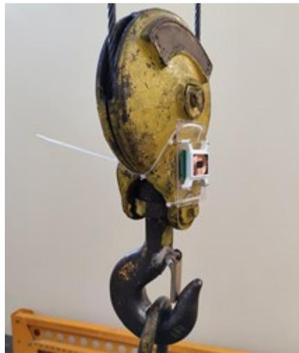
Figure 34. EDI+ZAPUNI real-time wireless sensor deployed on a crane.
