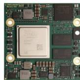
Figure 6. Enclustra Mercury XU5 platform
