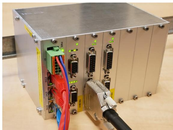
Figure 7: BB1 box with all I/O cards for Pilot 1, connected one encoder for test.
