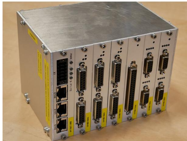
Figure 8: BB1 box with all I/O cards for Pilot 2.
